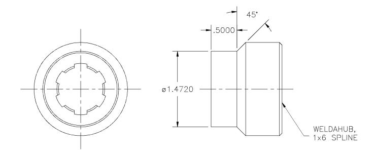
REV A: ELIMINATED RELIEF CUT AND CHAMFER ON LEFT SIDE 10/13/05
